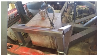
Sample Gas tank protector: Note ALL components must be 4" from sheet metal.
